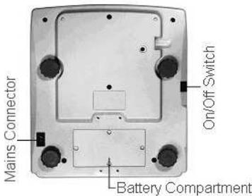
Attach the power cable to the connector on the base on the left of the scale. Plug in the power cable to the mains. Switch on the power switch located on the base on the right side of the scale.
